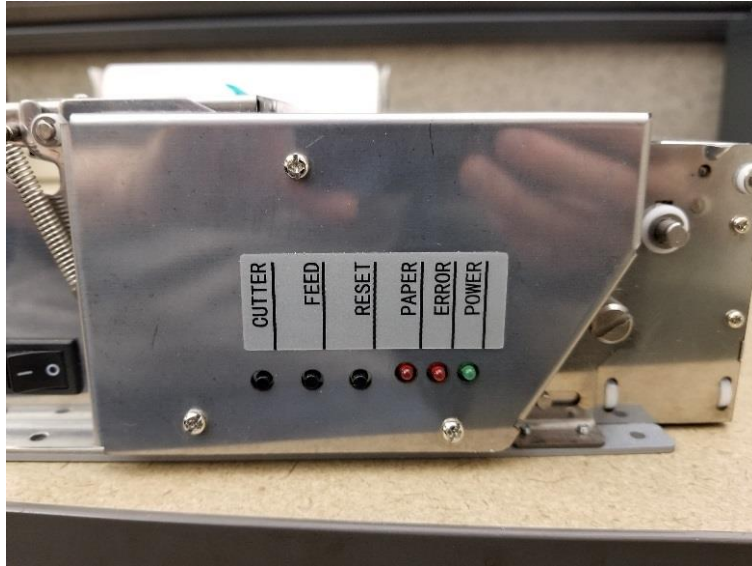
CUTTER, FEED, and RESET buttons. PAPER, ERROR, and POWER LEDs also pictured.
