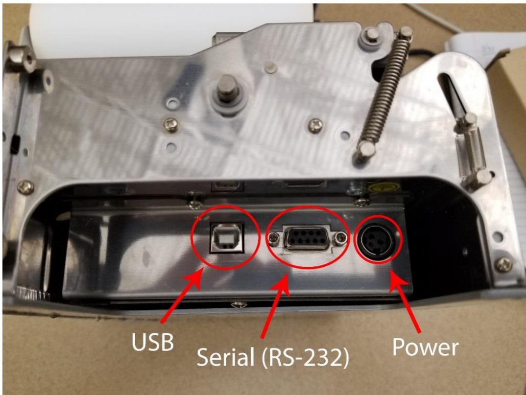
Ports on USB/Serial model
